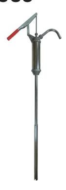
STM DA490S Lever Action Drum Pump is designed for transferring low viscosity lubricants, solvents, agricultural and industrial chemicals, additives and corrosive liquids. Pump is equipped with a self-adjusting telescoping suction tube for pumping fluids from 30 to 55 gallon (57, 114 and 208 litre) drums. Pump is self-priming and is designed to thread into a 1–1/2" or 2" drum.
