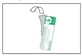
Stick the seal covering both the AIVIA door and chassis
