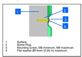
The screw head and washer together must not exceed 8 mm (0,31 in) thickness.
