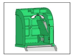
• Insert the 4 D-LR20 batteries supplied, respecting polarity indications on the bottom of the battery holder.
