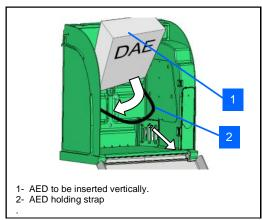
The strap allows the defibrillator to be easily removed in an emergency while ensuring that it is held properly.
