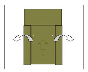
Put the template against the wall, with the arrow facing upwards and towards you.
